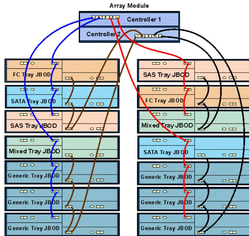
Array Module with Different Drive Tray Types
